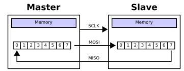
Using Enhanced SPI on Amped RF Wi-Fi Modules
